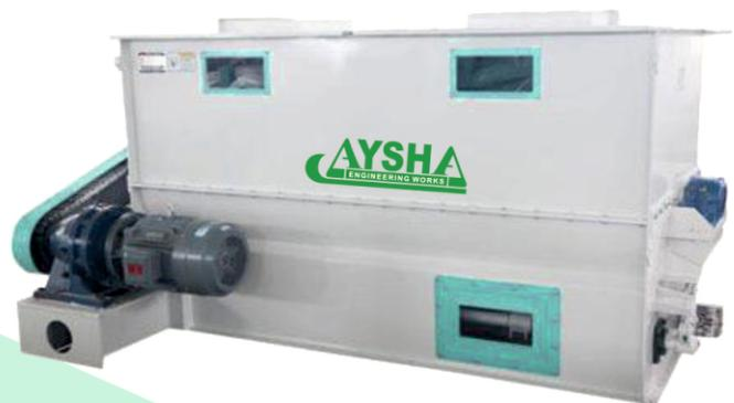
The central shaft is attached with geared motor. All bearings are of the universal flange cartridge type which are known for their lifetime lubrication.
